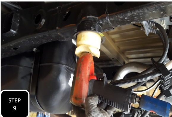
Step 9 Remove both rear bump stops from the frame.
