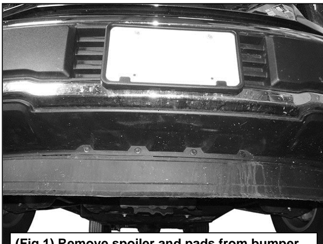
(Fig 1) Remove spoiler and pads from bumper
