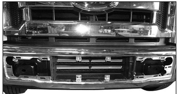
(Fig 2) Remove license plate. From behind bumper, release metal clips attaching plastic bumper pad to the bumper
