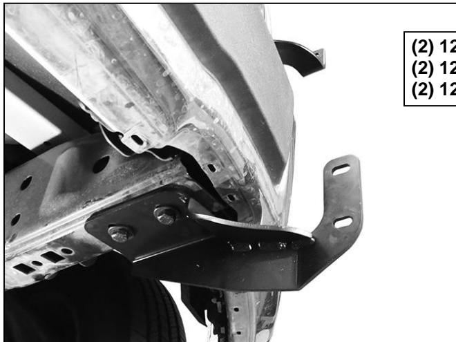
(Fig 8) Attach Frame Bracket to Nut Plate.
