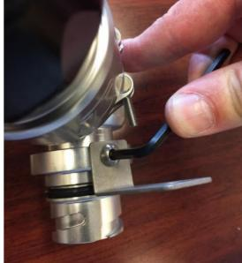
13. Screw the supplied intercooler adapter in place until it reaches home. Ensure that the O-ring (32.92x3.53) is installed on the adapter.
