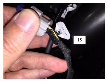
The scotch locks should look like this when installed correctly. Scotch locks are removable if the factory BOV is to be re-installed. Secure plug by using the supplied cable ties.
