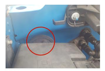
**STEP 10** // Optional LED light wiring, Route the on/off switch to the interior of the vehicle using a suitable body grommet. Mount the switch in the desired location. Zip tie any extra loose wiring away from heat and/or moving engine components.
