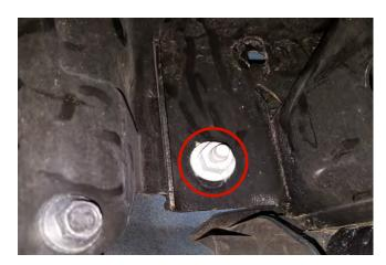
**STEP 3** // Unplug the factory fog light connectors and unclip the wiring harness from the bumper. Remove the lower (2) 21mm nuts. Then remove the front bumper from the vehicle. \*\*Note: Factory hardware will be reused.
