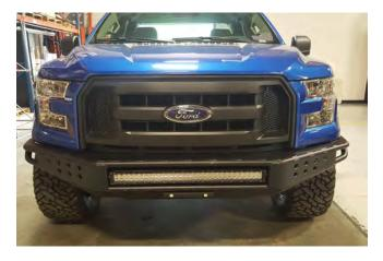
**STEP 7** // Slide bumper into place, and secure using the factory hardware.
