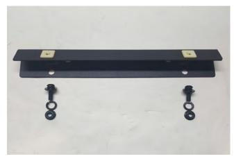
**STEP 4** // Attach the front license plate bracket to the new Barricade bumper if a front license plate is required using the (2) M6 screws, lock washers, and nuts.
