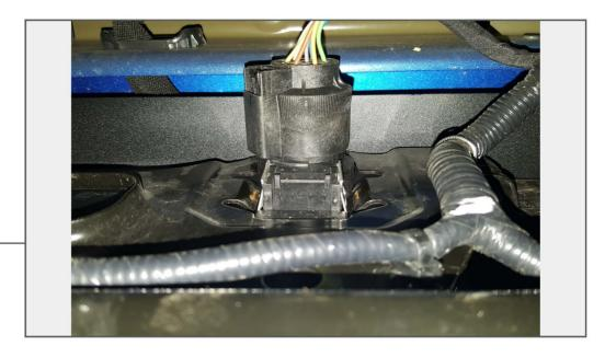
Unplug the factory license plate light harnesses and trailer plug connector, if equipped.
