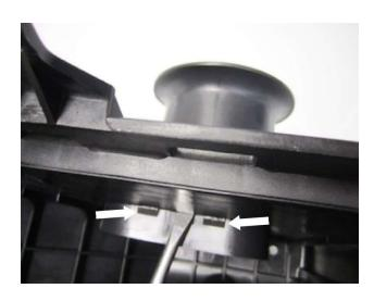
Install the Fender Inlet (W) into the factory intake box by pushing in firmly until it snaps into place.
