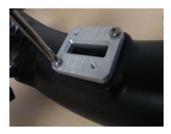
Install the MAF sensor using the 8-32 Screws (Q) and Rubber Washers (R) onto the MAF Plate (O).
