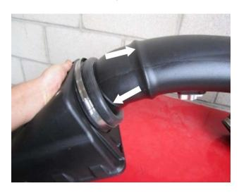
Tighten Hose Clamp #104 (D) on the Rubber Cuff (C). The rubber cuff will allow some movement of the tube to accommodate engine vibrations.
