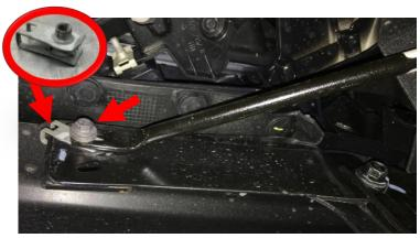
**3.** Remove the upper bolt that attaches the bumper end to the OE bracket and set aside. This bolt will be re-used for the install.
