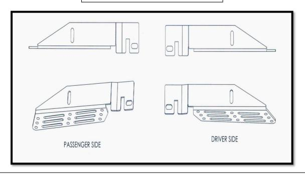
**5.** Install the driver side bracket using the OE bolt that was removed in **(step-1)** and the supplied M8x20mm Hex head and flanged nut. The OE bumper brace will be attached to the outside of the LED bracket. Leave loose at this time. **Note: It may be easier to install lights on bracket before installation.**
