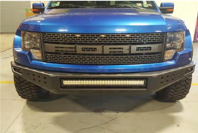
**STEP 6** // Slide bumper into place, and secure using the factory hardware.
