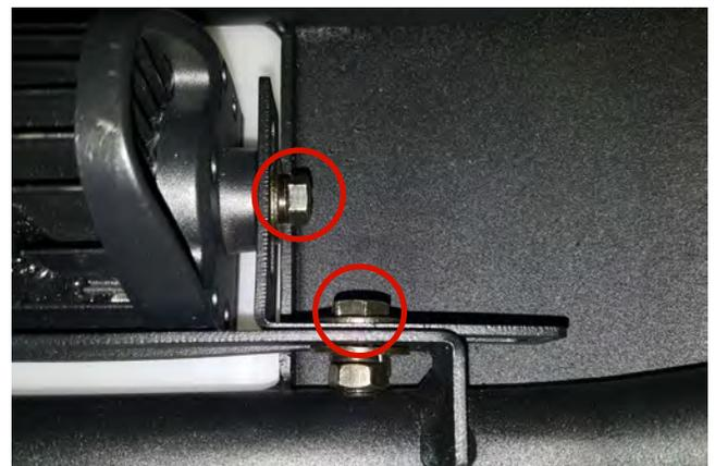
**STEP 4** // If purchased with the LED lighting option, install the LED light using the hardware provided in the light packaging. If choosing not to use the LED lighting. The bumper will include a bolt on mesh cover. Secure the cover to the bumper using (4) M8 x 20mm bolts, lock washers, and nuts.
