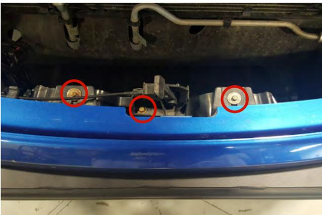
**STEP 7** // Re-attach and secure the (2) 8mm screws, and (1) 10mm bolt that hold the hood latch plate to the factory bumper lip.
