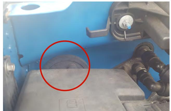
**STEP 10** // Optional LED light wiring, Route the on/off switch to the interior of the vehicle using a suitable body grommet. Mount the switch in the desired location. Zip tie any extra loose wiring away from heat and/or moving engine components.
