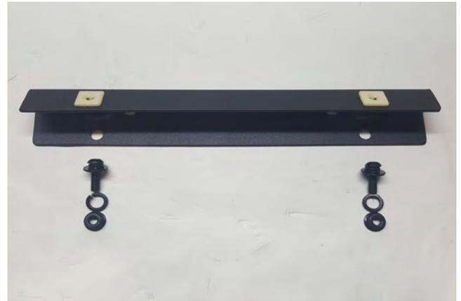
**STEP 3** // Attach the front license plate bracket to the new Barricade bumper if a front license plate is required using the (2) M6 screws, lock washers, and nuts.
