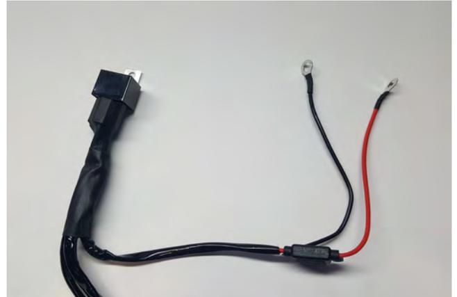
**STEP 9** // Optional LED light wiring, Install the Red 12+ volt wire to the positive battery terminal. Connect the black ground wire to the negative battery terminal. Mount the fuse in a safe location away from any damage that could occur. Tuck away any extra wiring.
