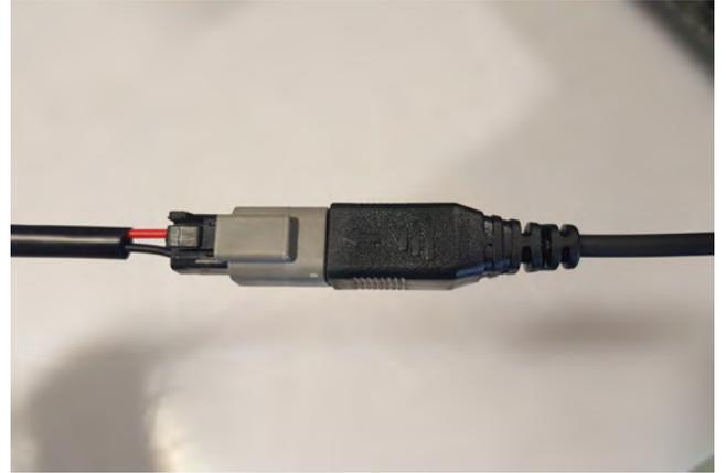
**STEP 8** // Optional LED light wiring, connect the (1) LED light bar into the supplied harness. Be sure to zip tie the access wiring away from any damage that could occur.
