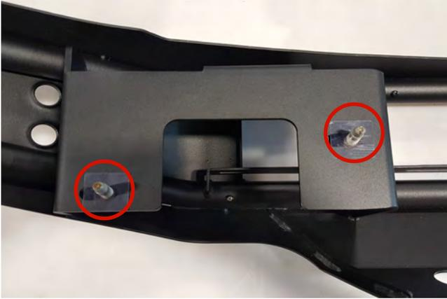
**STEP 5** // Using the supplied (4) plastic washers attach the factory bolts to the Barricade bumper.
