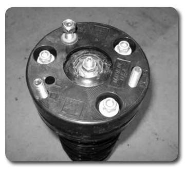
15. Tighten the factory strut hardware to 35 ft-lbs.. Figure 9
