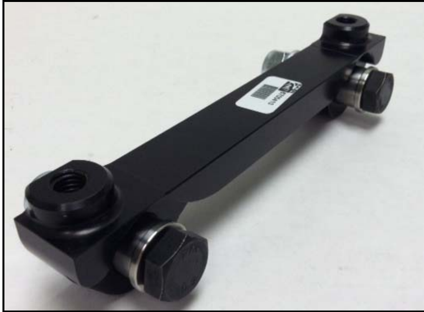
Figure 6: Bolts installed with nuts, washers and slider pins. Bolts enter the inboard side of the park assembly, then the slider pins, bracket, washers and nuts. No washers are required under the bolt heads.
