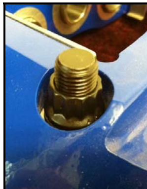
Figure 10: ARP studs, washers, and nuts installed
