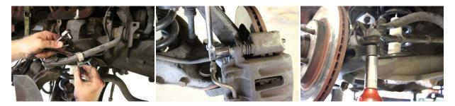
17. Depending on the year of the vehicle, you may have to grind down the front lip of the lower control arm about ¼". Grind smooth, then paint to protect the raw metal of the arm.
