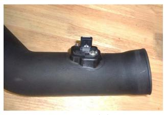
17. Place the MAF sensor gasket (12) over the sensor, ensuring correct orientation. Then install the sensor in the intake tube, using M4 screws (13).
