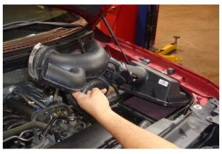
8. Separate the intake duct from the throttle body, then remove the assembled duct and airbox cover from the vehicle. Remove the stock air filter.
