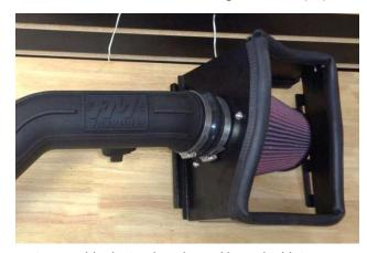
18. Assemble the intake tube and heat shield. Snug the tube clamp (do not tighten at this time).
