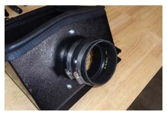
13. Slip the 2 larger screw clamps (10) onto the flex coupler (11). Install the large end of the coupler onto the air filter adapter, pushing it flush against the heat shield. Tighten only the filter adapter clamp at this time. (Leave the other clamp loose.)
