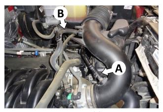
5. On the PCV hose connector (A), release the latch and disconnect the hose from the intake duct. Disconnect the EVAP hose (B) from both the intake duct and the check valve.
