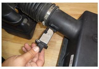
Remove the MAF sensor from the airbox cover, then remove the stock gasket from the sensor.
