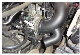
6. Loosen the screw clamp securing the air intake duct to the throttle body.
