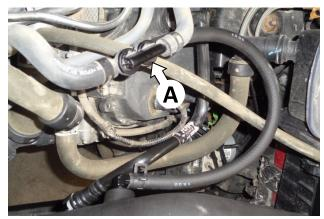
21. Push one end of the 3/8" hose (17) onto the EVAP check valve (A). Route the hose to the barbed elbow as shown and cut it to length. Push the hose onto the elbow, and secure it with the pinch clamp (16).
