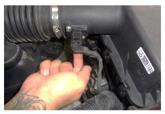
4. Disconnect the mass airflow (MAF) sensor plug by pulling the locking tab (on the bottom of the plug) away from the sensor until it stops, then pulling the plug straight off the sensor.
