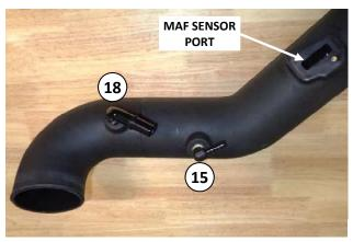
15. Apply 2 wraps of nylon thread tape to the threads of the 5/8" quick connect elbow (18) and the 3/8" barbed elbow (15). Install the elbows in the intake tube (14), oriented approximately as shown.
