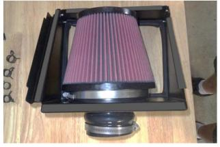
14. Slip screw clamp (3) onto air filter (2), then install the filter on the filter adapter and tighten the clamp.
