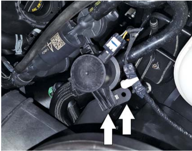
14. Reinstall the two (2) push pins into the dirty air inlet.
