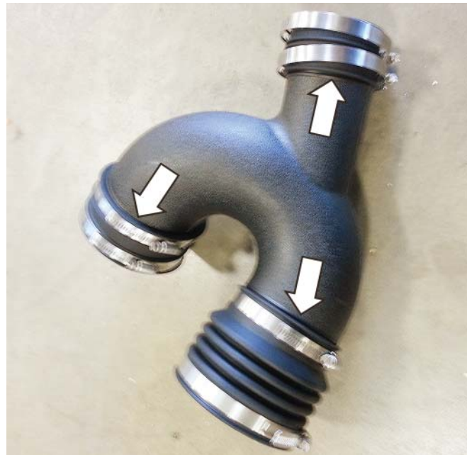
12. Install the clean air tube assembly between the throttle body and the air box. Tighten the clamps to 3 Nm.
