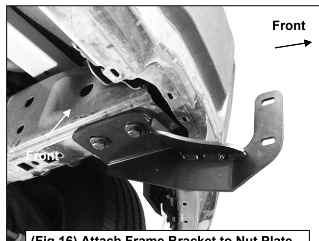
(Fig 16) Attach Frame Bracket to Nut Plate.
