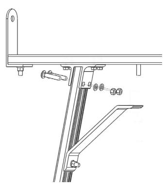
Slide the HD brace along the leg towards the load bar. Align the 3/8"-16 x 1-3/4" bolt in the load bar with the top bolt hole on the HD brace. Loosely secure the HD brace with a 3/8"-16 nut and a 3/8" split lock washer. Repeat for other legs.
