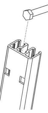
Install the HD brace to the leg by placing the HD brace on the 3/8"-16 x 1-3/4" bolt in the leg. Loosely secure with a 3/8"-16 nut and a 3/8" split lock washer. Repeat for other legs.
