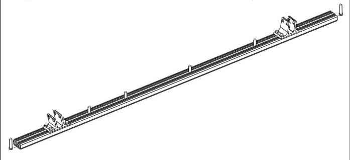
Install the load secure posts as shown. Place the end load secure posts so they are flush against the load bar.
