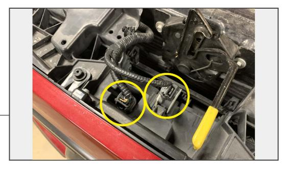
Disconnect the (2) electrical connectors next to the hood latch.
