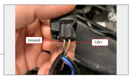
**Lighting if equipped:** Route the grille light wiring to the passenger side headlight. Tap into the parking light connector using (2) provided Scotch-Locks following the diagram below. Confirm lighting works before re-assembly.
