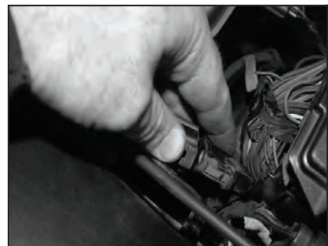
Step 7 Disconnect the MAF sensor from the harness and remove the assembly from the housing.
