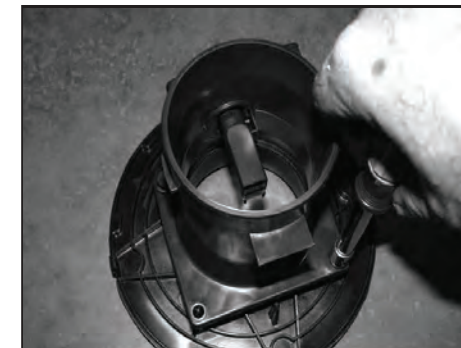
Step 14 Remove the MAF sensor assembly from the housing.
