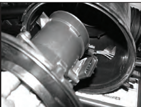
Step 7 Disconnect the MAF sensor from the harness and remove the assembly from the housing.
