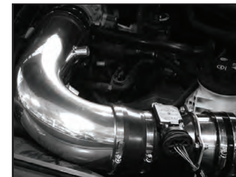
Step 17 Install the 4"-3.5" coupler and the 4" coupler onto the MAF sensor assembly, install the unit onto the intake tube and reconnect the wiring harness. Note that the sensor must be located at the top of the assembly and the arrow on the MAF sensor must point towards the throttle body.
