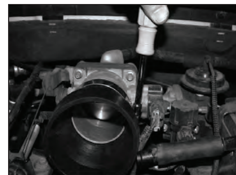
Step 10 Attach 4"-3" coupler to the throttle body and secure.
