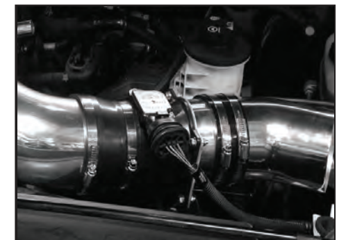
Step 18 Install the short aluminum intake tube into the 4"-3.5" coupler. Slide the arm under the power steering reservoir and tighten the three bolts for the reservoir.
