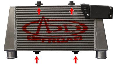
35. Using a 13mm Socket and the OEM bolts you removed in Step 13, install the supplied lower intercooler support. (Fig AJ)
