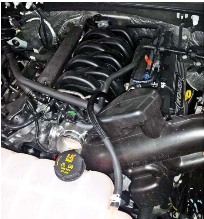
9. Remove the two (2) push clips retaining the dirty air inlet duct to the grill closeout.
