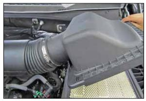
4. Release the locking clips that secure the upper air filter housing to the lower housing, then lift the upper housing and remove it from the vehicle. Remove the factory air filter from the vehicle. 5. Loosen the two hose clamps that secure the factory intake tube to the turbo inlets, then remove the factory intake tube from the vehicle. NOTE: K&N Engineering, Inc., recommends that customers do not discard factory air intake.
