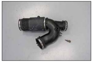
15. Remove the inlet temperature sensor from the factory intake tube.
