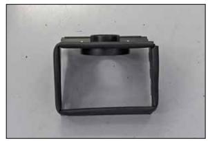
9. Install the K&N<sup>®</sup> filter adapter into the heat shield and secure with the provided hardware.
