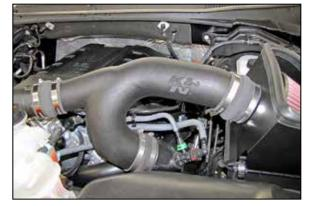
17. Install the K&N<sup>®</sup> intake tube into the couplers at the turbo inlet tubes and then into the coupler at the filter adapter, adjust the tubes for best fit and then secure with the provided hose clamps.
