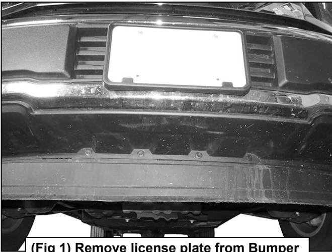
(Fig 1) Remove license plate from Bumper
