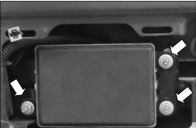
(Fig 3) Remove and unplug adaptive cruise control from driver/left side of frame, if equipped
