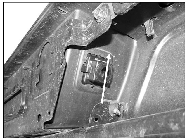
(Fig 2) Unplug license plate lights
