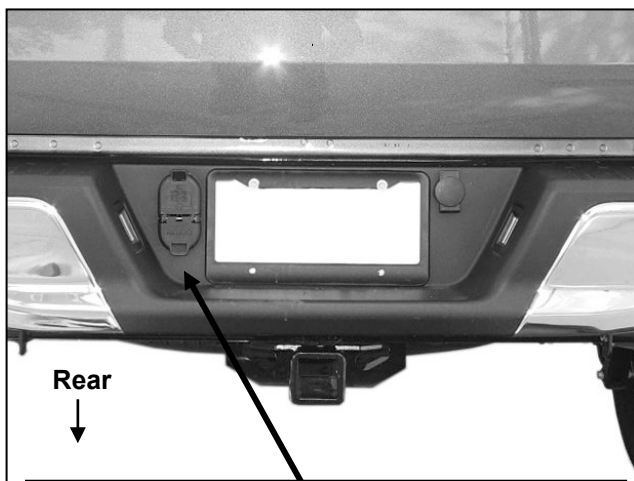
(Fig 1) Unplug and remove 7-wire trailer plug
