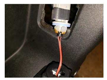
**Step 3\\**Plug the new Axial light harness into the factory light bulb socket. \*\*Note: Test lights for proper function at this point. If the light is not working, unplug the harness from the socket and rotate 180 degrees and test light again.
