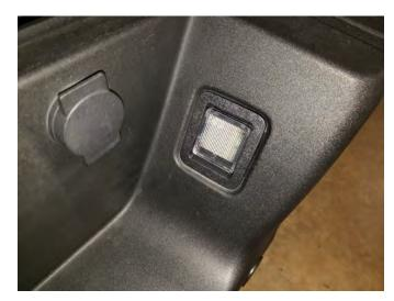
**Step 4\\**Install the new Axial license plate light until it clicks in place. Installation is now complete.
