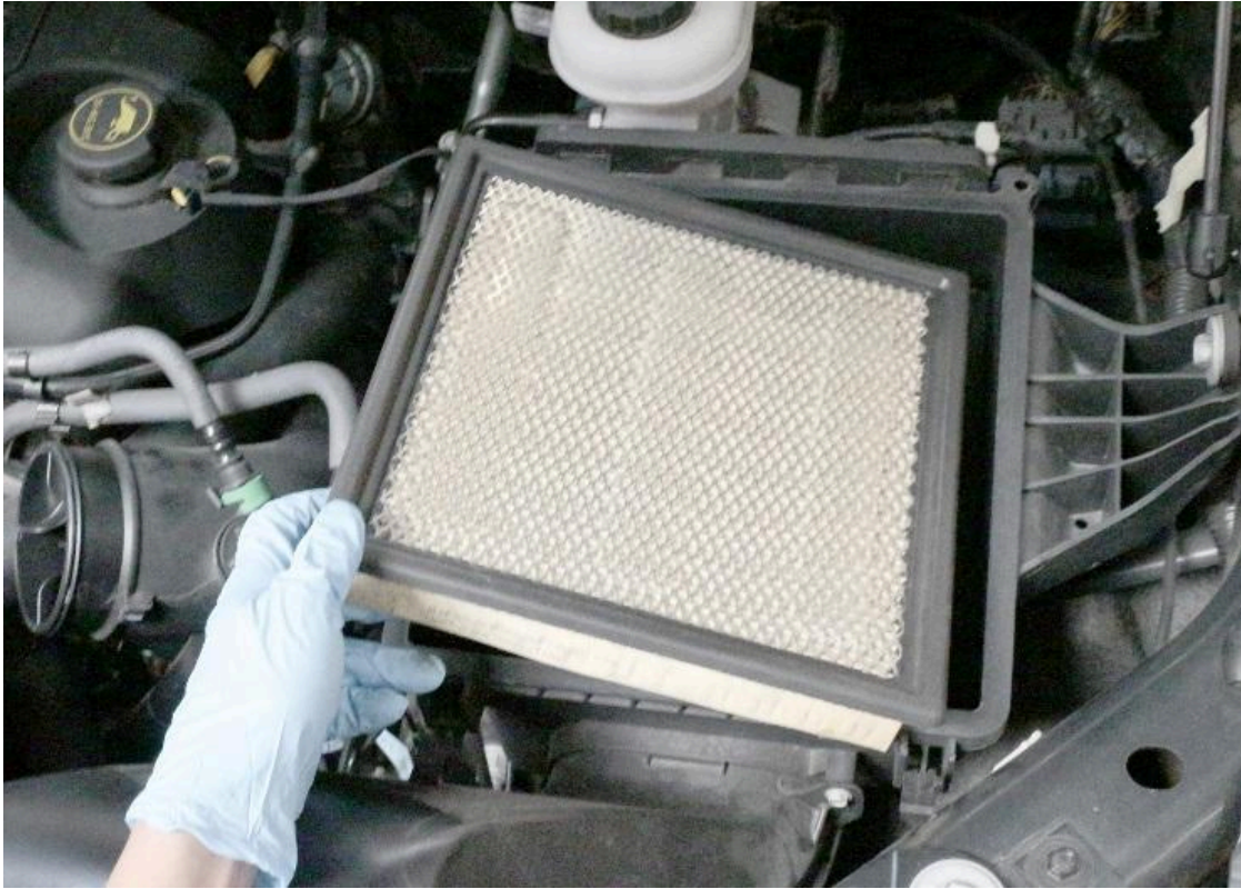
6. Remove the air filter from the lower air box.
