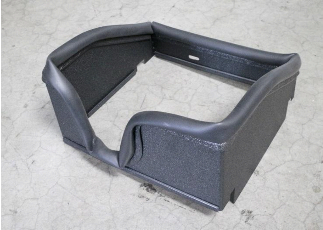
8. Install the bubble edge trim along the upper perimeter of the heat shield.
