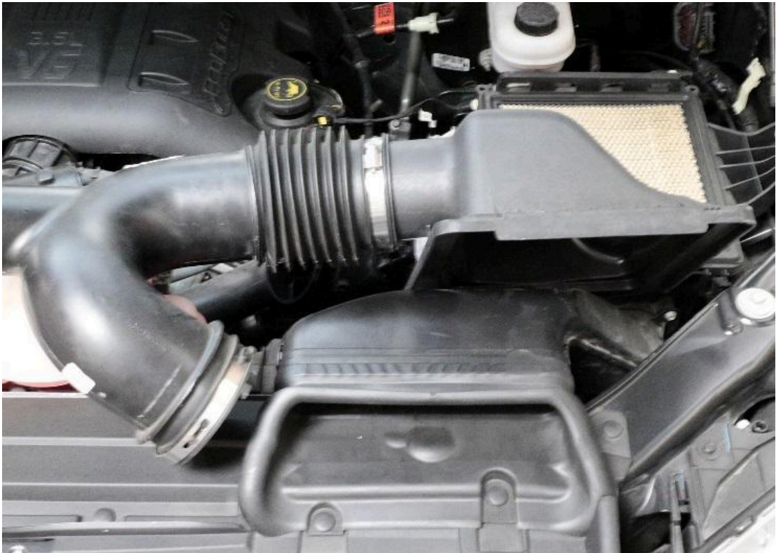
5. Remove the air intake tube and upper air box from the engine bay.
