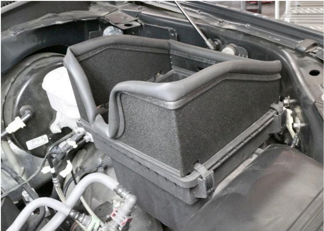
11. Place the heat shield onto the lower air box. Be sure to line up the two tabs at the front and rear.
