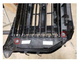
**STEP 9** // Separate the grille from the base by removing the (2) 10mm lock nuts on each side of the grille. Then remove the (3) 10mm nuts across the bottom. The grille will now separate from the base. \*\*Note: Hardware will be reused.
