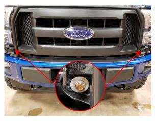
**STEP 7** // Locate, and remove the lower (2) 8mm bolts securing the grille to the vehicle. Grille will now be free, carefully pry the factory grille away from the vehicle. \*\*Note: Hardware will be reused.
