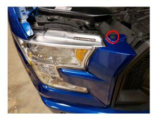
**STEP 2** // Using a trim panel removal tool, remove the push clip securing the upper headlight bezel in place.
