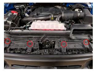
**STEP 5** //Locate, and remove the upper (4) 10mm screws securing the grille to the vehicle. \*\*Note: Hardware will be reused.
