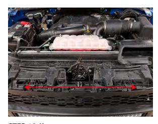
**STEP 12** // Using the hardware from steps 5 & 7, install the grille to the vehicle. \*\*Note: Be sure to align the grille in the center position of the headlights.
