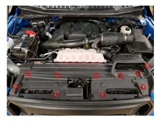
**STEP 1** // Begin by locating the (10) plastic push clips securing the factory radiator cover, and remove using a trim panel removal tool.
