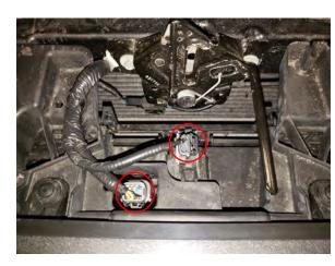
**STEP 4** // Carefully unplug the wiring connections for the grille's shutter system to the factory grille.
