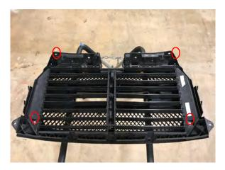
**STEP 11** // Install the new grille to the factory base by using the provided (4) speed clips and using (4) 10mm nuts previously removed. \*\*Note: Make sure the (5) LED harnesses are not in between grilles.
