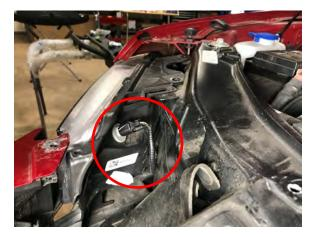
**STEP 13** // To wire the LED lights, find the marker light harness on the top of the headlight. Connect all 3 LEDs to the included wiring harness, then splice into the marker light harness and attach the red wire to positive and black to negative.
