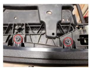
**STEP 8** // The factory grille is two pieces. Remove the (2) push clips on each side (4) total across the top of the grille and base.
