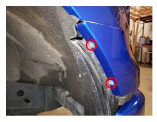
**STEP 3** // Locate, and remove the (2) 7mm screws holding the headlight bezel to the splash shield.
