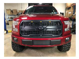
**STEP 14** // Reinstall the headlight bezels, and radiator cover in reverse form.
