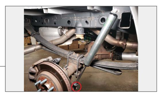
Install the new shock using the original hardware. If equipped, ensure any valving is easily accessible and will not interfere with any other suspension components. Torque shock fasteners to 66 ft. lbs. Reinstall the fender liner and reinstall wheels torque to 150 lb. ft. Installation is now complete.
