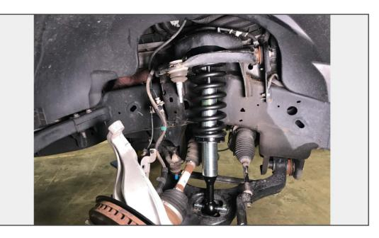
Install the coilover assembly. Rotate the upper strut mount as needed to align the mounting holes. Torque upper nuts to 52 lb. ft. and install the lower bolts and torque to 66 lb. ft.
