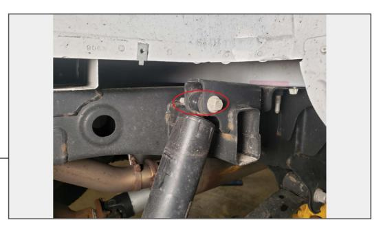
With the fender liner removed, locate the upper shock mount. Remove the upper shock bolt using a 15mm & 18mm socket and ratchet.
