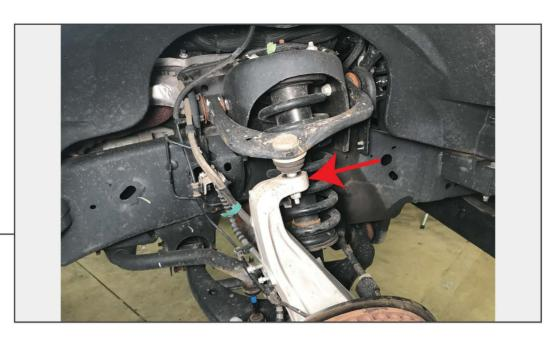
Using a 18mm socket, loosen the nut securing the upper ball joint to the knuckle. Using a sledge hammer, strike the knuckle to separate the ball joint from the knuckle. Remove the nut to separate the control arm from the knuckle. This will allow additional space when removing the strut assembly from the vehicle.
