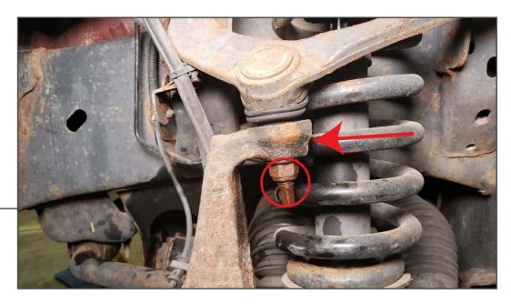
Using a 18mm socket, loosen the nut securing the upper ball joint to the knuckle. Using a sledge hammer, strike the knuckle to separate the ball joint from the knuckle. Remove the nut to separate the control arm from the knuckle. This will allow additional space when removing the strut assembly from the vehicle.
