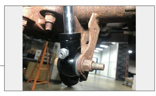
Install the new shock on the axle using the original hardware. If equipped, ensure any valving is easily accessible and will not interfere with any other suspension components.
