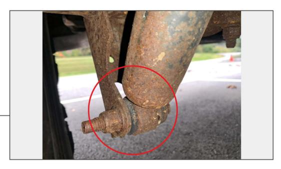
Locate the lower shock mount. Remove the lower shock bolt using a 15mm & 18mm socket and ratchet. Remove the shock from the vehicle.
