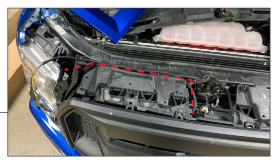
Feed the LED light wiring harness through the grille support and route the harness to the right side headlight. Ensure the wiring doesn't get pinched under the radiator cover.
