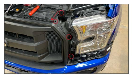
Remove the (3) plastic clips that hold the rubber air dam to the grille surround. Then remove the (2) 10mm fasteners that hold the grille to the vehicle. Repeat the process on the other side.
