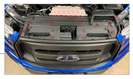
Using a panel removal tool or flat blade screw driver, remove the (10) clips holding the radiator cover to the vehicle.
