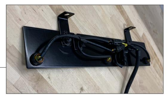
Assemble the LED light bracket using the (2) "L" brackets, (2) M6 bolts, (2) flat washers, and (2) lock nuts. Ensure the wiring is secured to the wiring clips to prevent it from hanging below the light. Grille configuration will determine which mounting holes are used. Test fit the light and adjust as needed.
