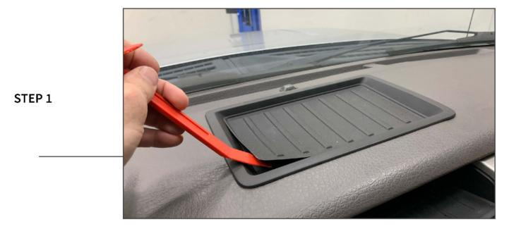
Using a plastic pry tool, remove the factory rubber mat from the upper dash tray.
