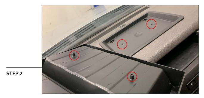
Using the locating pins, install the tray onto the factory tray. The pins will locate and prevent the storage bin from moving.
