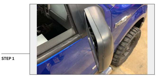
While wearing gloves, carefully remove the mirror glass. Tilt the glass down so that the top edge is accessible.
