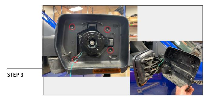
Using a T20 Torx bit, remove the (4) screws that secure the mirror shell to the vehicle. Pull the shell away from the mirror housing.
