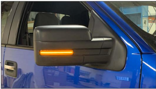
Test the light by turning on the respective turn signal. Once the light is confirmed working, follow steps 1-3 in reverse order to complete the install.
