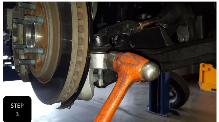
Step 3 Unbolt the tie rod from the spindle and break it loose by hitting the side of the spindle, right at the tie rod, with a hammer. NOTE: NEVER HIT THE TIE ROD ON THE THREADS.
