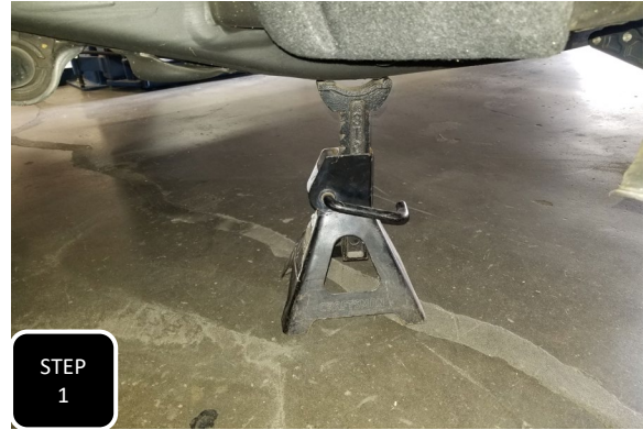
Step 1 Jack up the front of the truck and support under the frame with jack stands.
