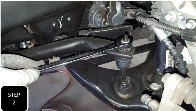
Step 2 Unbolt the sway bar end link from the sway bar.
