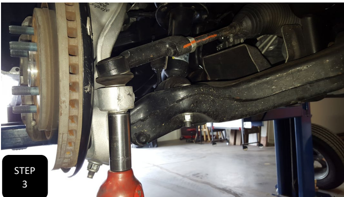
Step 3 Unbolt the tie rod from the spindle and break it loose by hitting the side of the spindle, right at the tie rod, with a hammer. NOTE: NEVER HIT THE TIE ROD ON THE THREADS.
