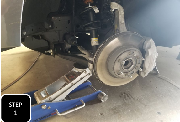
Step 1 Jack up the front of the truck and support under the frame with jack stands.
