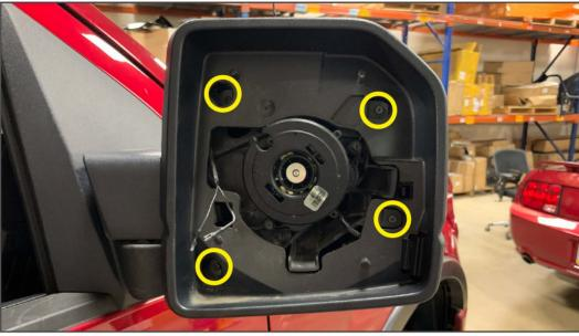
Using a T15 Torx driver, remove the (4) screws holding the mirror shell together.
