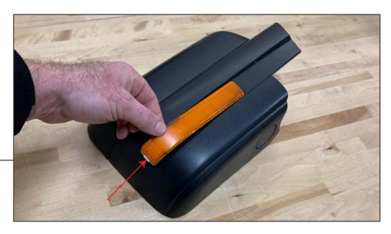
Remove the factory orange reflector from the outer mirror shell. Pry on the outer edge to unclip it from the housing.
