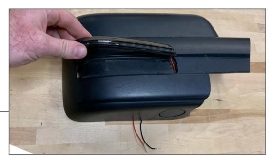
Pass the lights wiring through the mirror shell and clip the light into the mirror shell.
