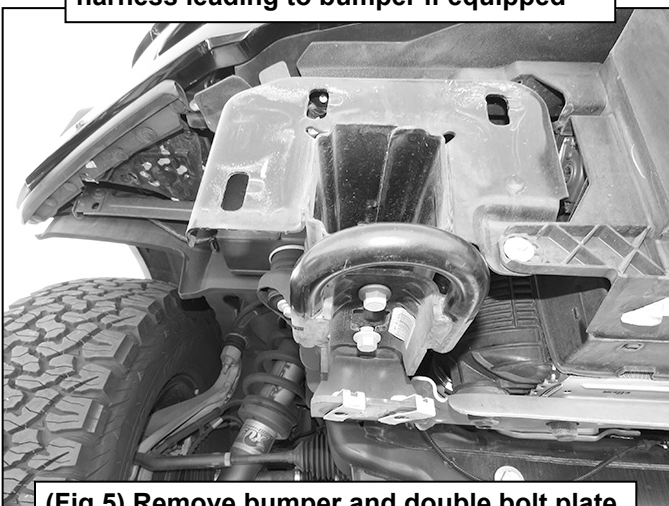
(Fig 5) Remove bumper and double bolt plate
