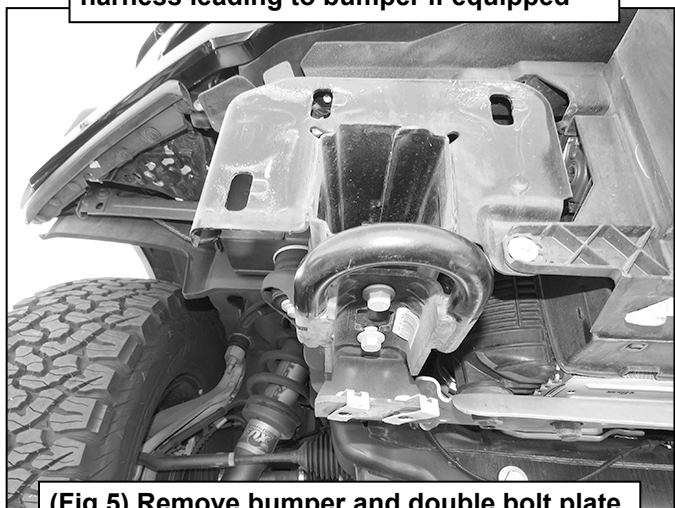
(Fig 5) Remove bumper and double bolt plate
