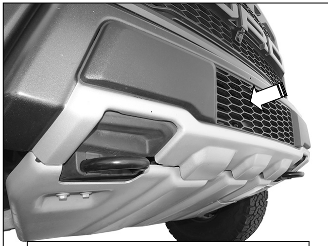
(Fig 1) Remove license plate, skid plate and plastic center pad (arrow) from bumper
