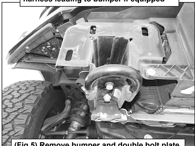
(Fig 5) Remove bumper and double bolt plate
