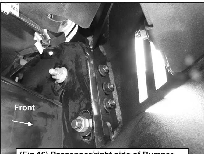
(Fig 16) Passenger/right side of Bumper attached to Bracket (pictured from below)
