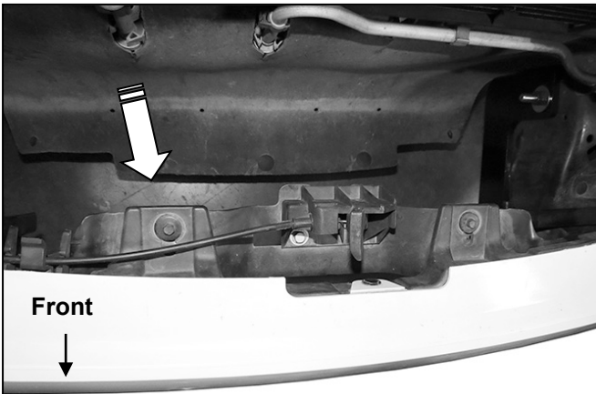
(Fig 7) Reattach metal bracket and hood latch to bottom of tabs on plastic fascia body panel
