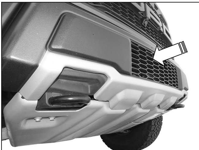
(Fig 1) Remove license plate, skid plate and plastic center pad (arrow) from bumper
