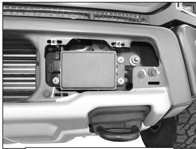
(Fig 2) Unplug and remove sensor if equipped (driver/left side pictured)
