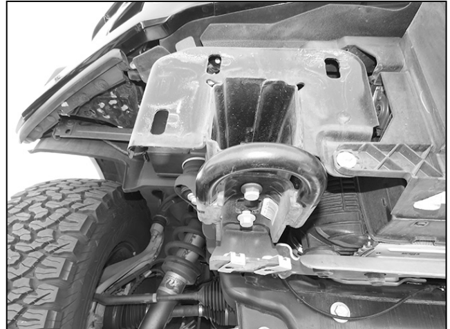
(Fig 6) Remove bumper and double bolt plate
