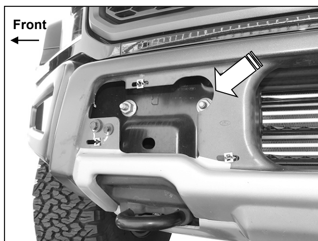
(Fig 4) Remove hex nuts (arrow) and remove bumper
