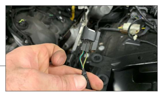
Using the supplied scotchlok connectors, connect the factory plug to the LED light harness as follows:
