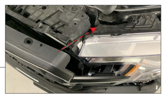
Install the grille so that the wiring harness exits the grille towards the driver's side headlight.
