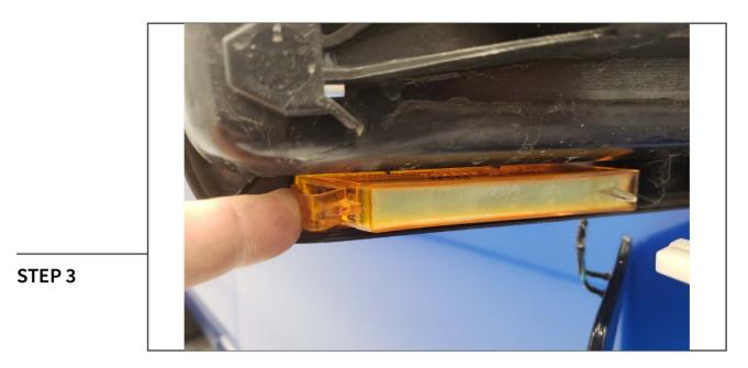
Unplug the wiring harness from the mirror light, and push in the tab to release the mirror light from the mirror base.
