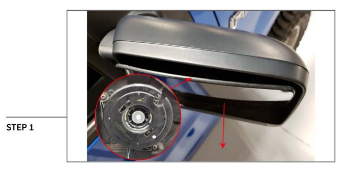
Begin by tilting the mirror full downward. Using a flat blade 0screw driver, gently depress on the clips holding the glass to the mirror housing. Then carefully pry the glass away from the mirror housing. The support mirror glass so that it isn't only hanging by the wires.
