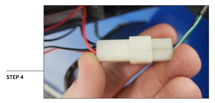
Connect the new Axial mirror light harness to the factory mirror light harness.
