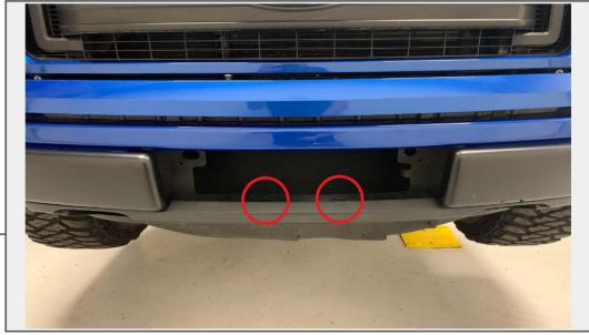
Begin by pushing the (2) bottom hooks into the lower portion of the bumper until there is an
