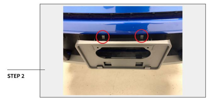
Pull down on the bracket enough to push the top of the bracket under the bumper. Once the bracket is pushed back, push up on the backside of the bracket to secure the (2) clips into the bumper. There will be an audible click to ensure it is secured.
