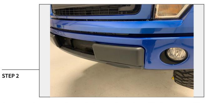
Push the guard into place, starting from the inside moving out. Once all (4) clips make an audilble click, installation is complete.
