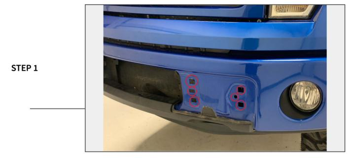
Using the designated guard, align the bumper guard with the pre-existing holes in the bumper.
