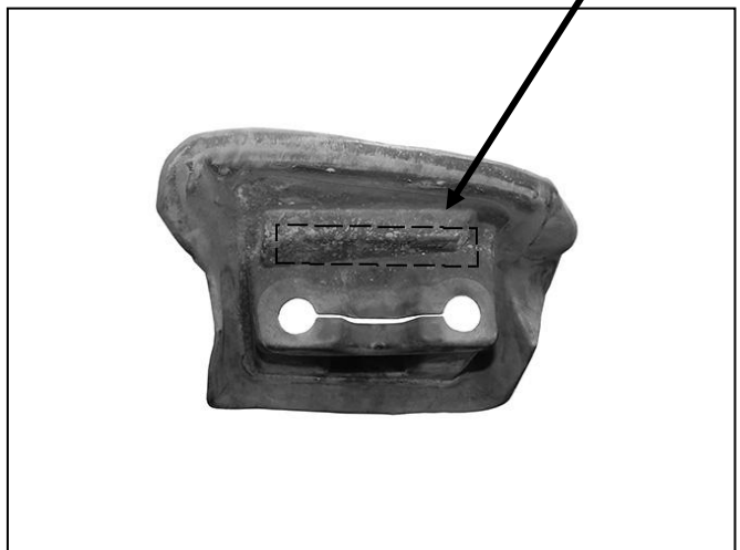
(Fig 8) Models with tow hooks, cut a slot from the rubber seal to clear the Support Brackets
