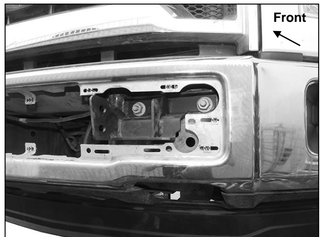
(Fig 4) Driver/left Frame Bracket installed
