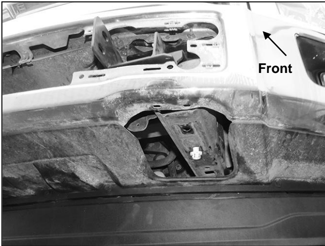
(Fig 5) Models with tow hooks, remove forward bolt, loosen but do not remove rear bolt to hold factory double nut plate in place in frame
