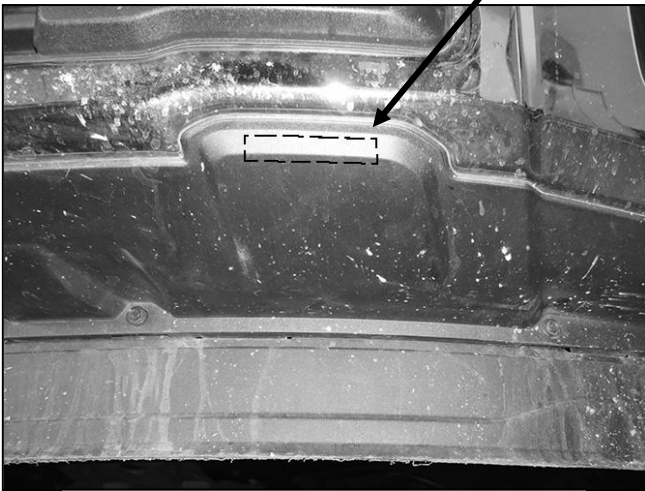
(Fig 11) Models without tow hooks, cut a slot from the plastic splash guard to clear the Support Brackets
