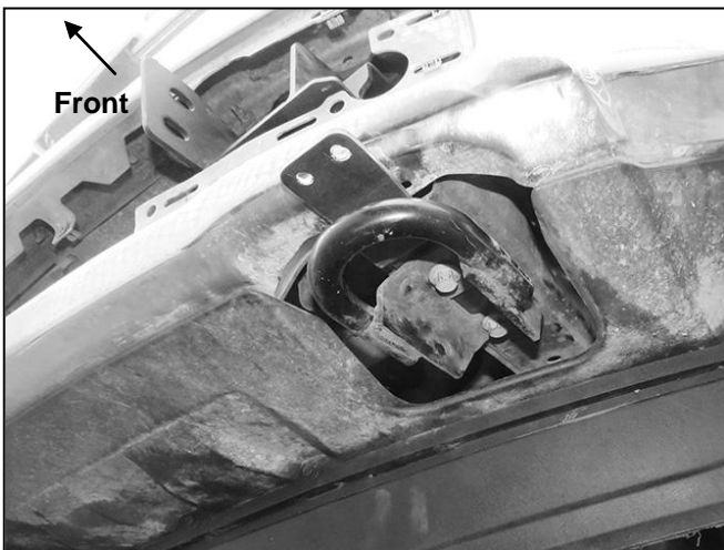
(Fig 7) Brackets installed, model with tow hook pictured
