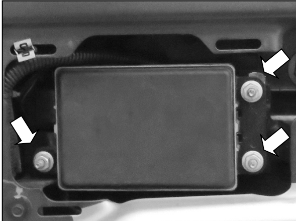
(Fig 3) Unplug and remove adaptive cruise control from driver/left side of frame, if equipped
