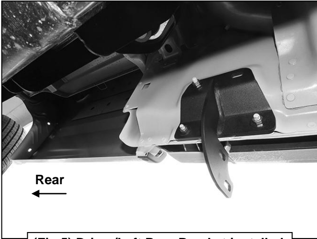
(Fig 5) Driver/Left Rear Bracket installed
