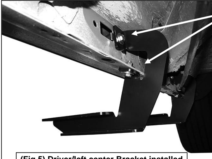
(Fig 5) Driver/left center Bracket installed
