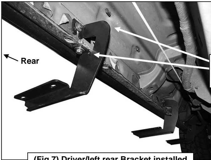
(Fig 7) Driver/left rear Bracket installed
