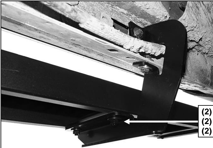
(Fig 10) Driver/left front Running Board to Bracket
