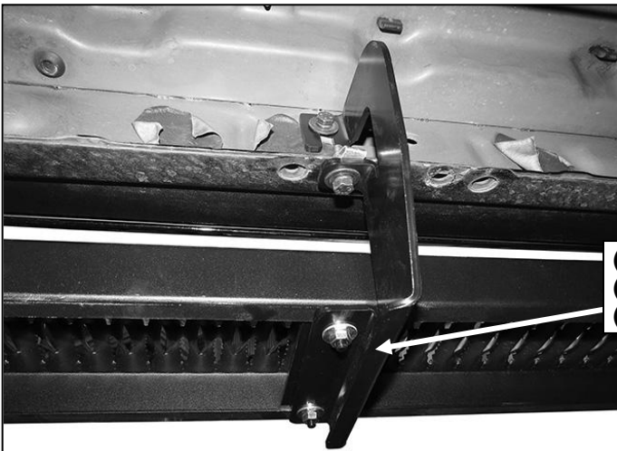
(Fig 12) Driver/left rear Running Board to Bracket
