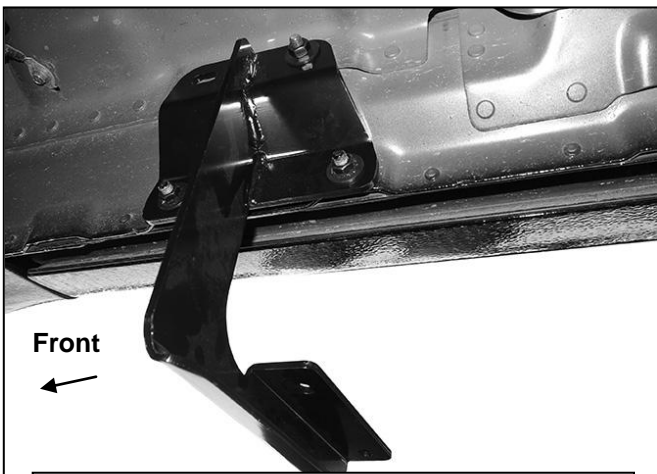
(Fig 5) Passenger/right front Bracket installed
