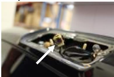
Remove the brake light bulb out
